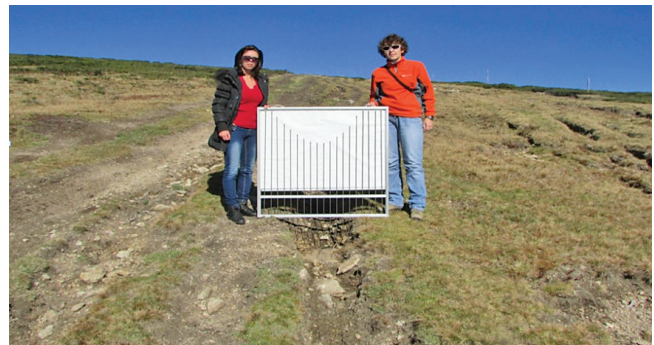
Fig. 3. Micro-topographic profiler for measuring cross sections of rills and small gullies
