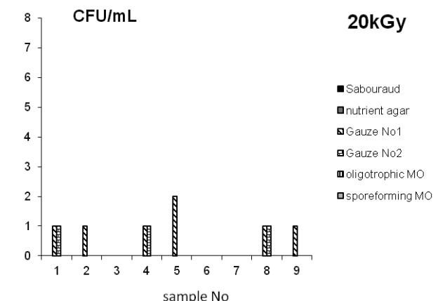
**Fig. 4. Quantity of microbial populations growing on different media after 20 kGy irradiation: Sabouraud – fungi, Nutrient agar – heterotrophs; Gauze 1 and 2 – starch assimilating microorganisms; no oligotrophic and sporeforming bacteria.**
