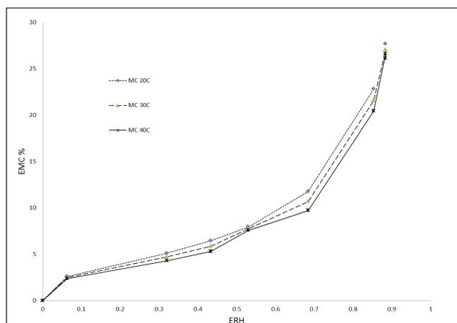
Fig. 1. Moisture sorption isotherms of Bermuda grass using Halsey model
