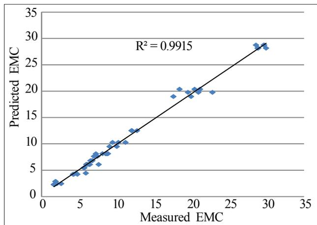
Fig. 2. Relationship between predicted and measured EMC for temperatures 20-40°C using ANN
