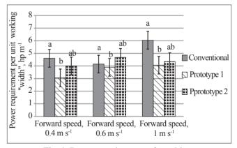
Fig. 1. Power requirement of machines
