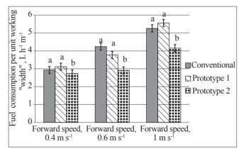
Fig. 2. Fuel consumption of machines
