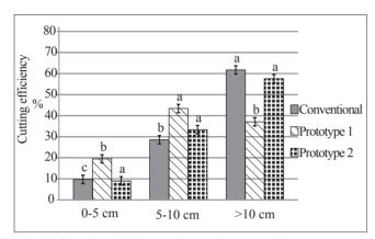
Fig. 3. Cutting efficiency of machines at a forward speed of 0.4 m s<sup>-1</sup>
