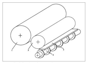
Fig. 3. 3D-view of the combing wool process
