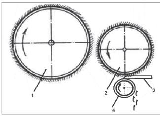
Fig. 2. General view of process of wool (canvas) transition from the main drum on a doffer drum
