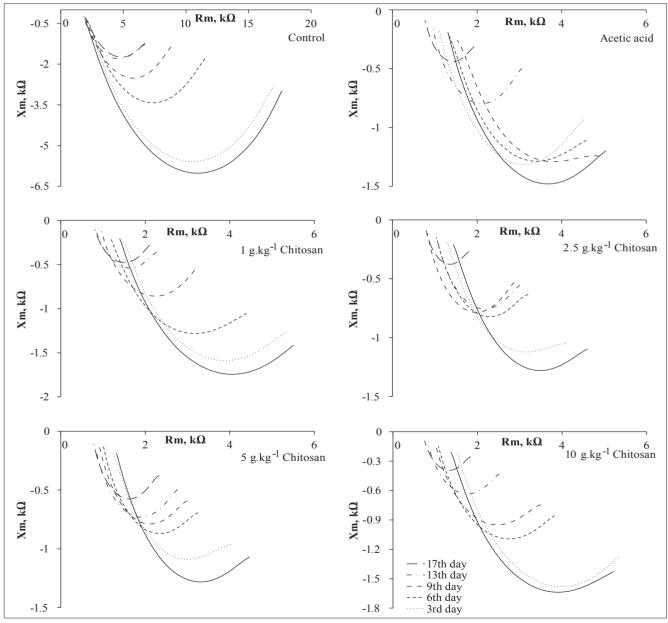
Fig. 2. Impedance changing of the coated apple cubes during the shelf-life time
