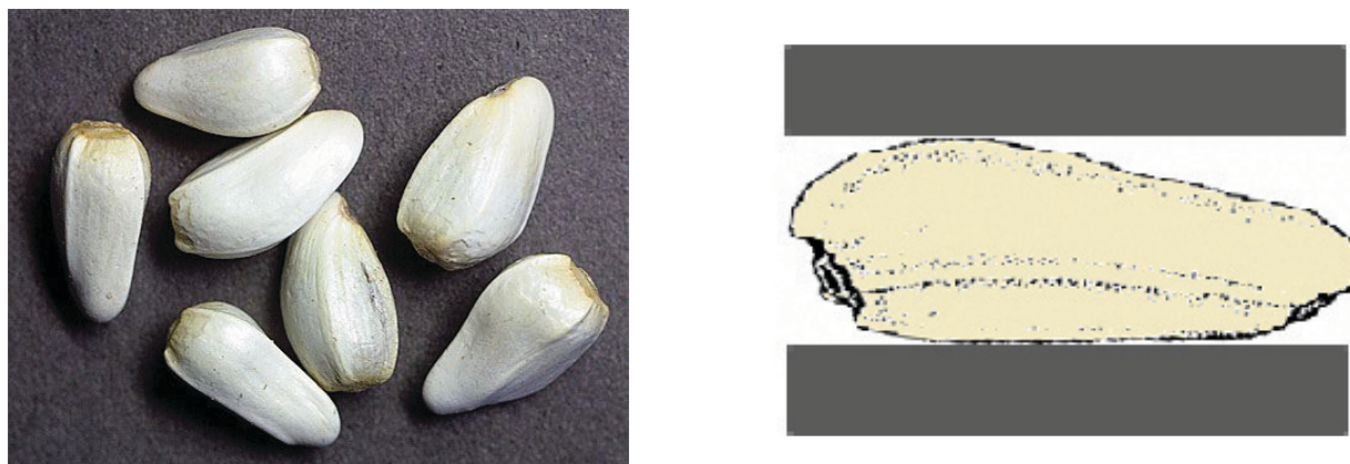
Fig. 1. a) A view of safflower seeds, b) Compression test of safflower seed (not to scale)
