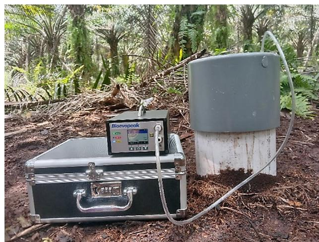
**Fig. 2.** Measurement of CO<sub>2</sub> emissions in the Experimental Plot using a Portable Infrared CO<sub>2</sub> analyzer
