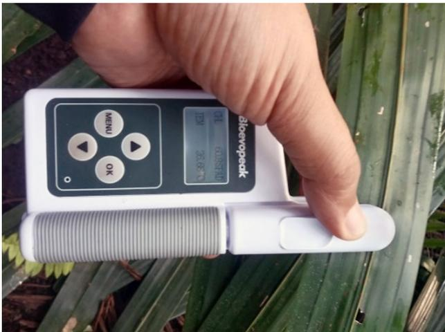
**Fig. 7. Measuring the greenness of leaves**
