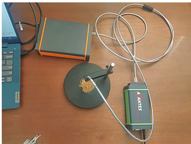
Fig. 1. Schematic diagram for measuring fluorescent spectra of opaque samples
