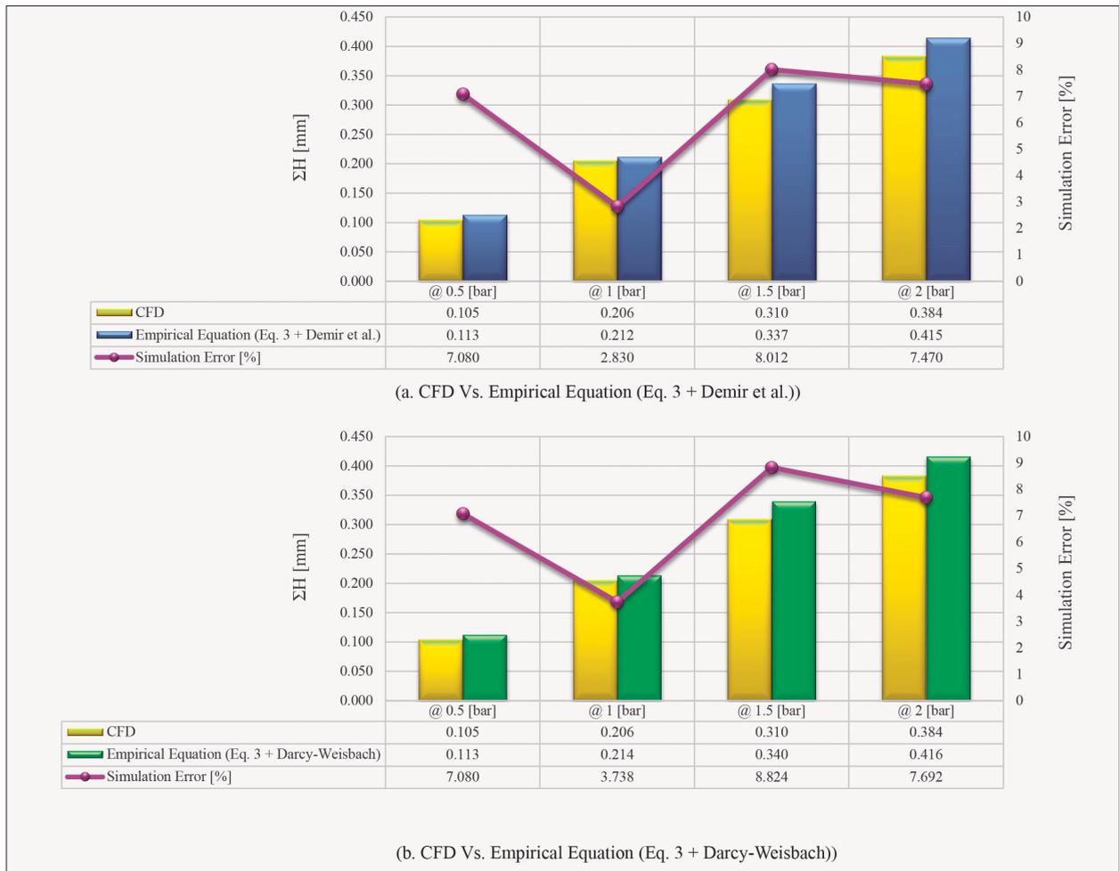
**Fig. 6. Comparison of the results obtained from empirical and CFD calculations**
