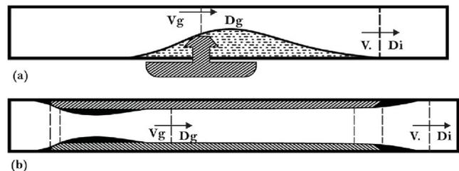
**Fig. 1. Schematic view of flow for (a) on-line, (b) integrated in-line emitters**
