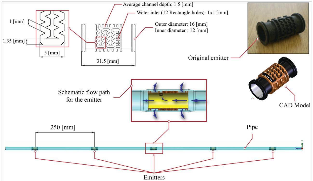
**Fig. 2. General specifications of the emitter and pipe**
