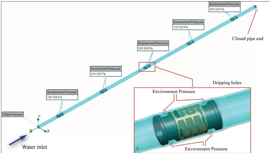
Fig. 3. Boundary conditions (Absolute Pressure)
