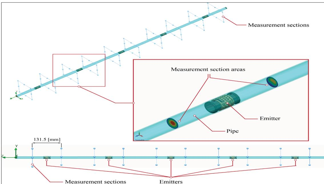
Fig. 4. Measurement section areas for velocity and pressure using CFD analysis
