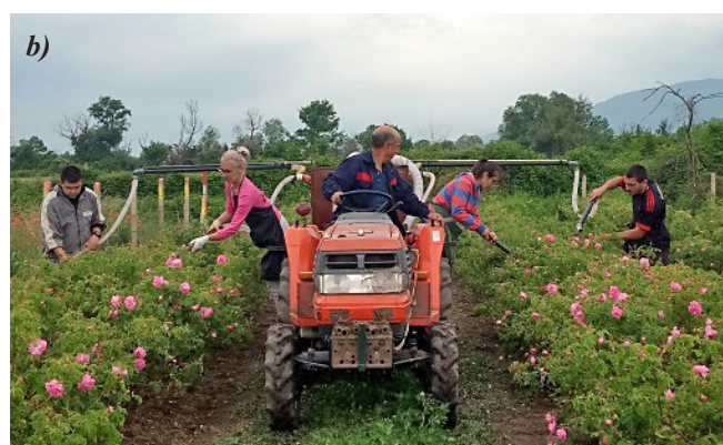
Fig. 2. Experimental testing in field conditions of the rose harvesting machine a – one-row variant RHM-1; b – two-row variant RHM-2
