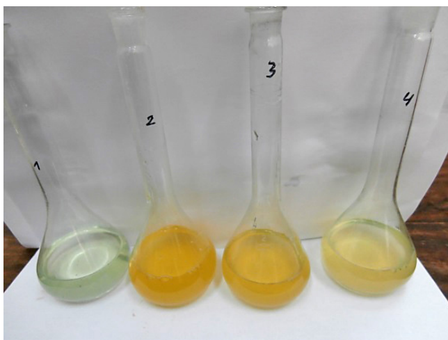
Fig. 1. Light bluish colouring of sample I: sugar syrup inverted with confectionery invertase, after adding Carrez I solution, in comparison with samples of bee honey
