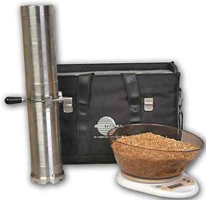
Fig. 1. Determination of the hectolitre mass with a feed meter
