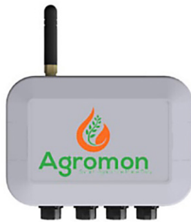
Fig. 2. Agromon Wireless Transmitter (WT-AGRO-3S)
