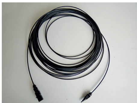
Fig. 3. Plastic fiber with a length of 10 m
