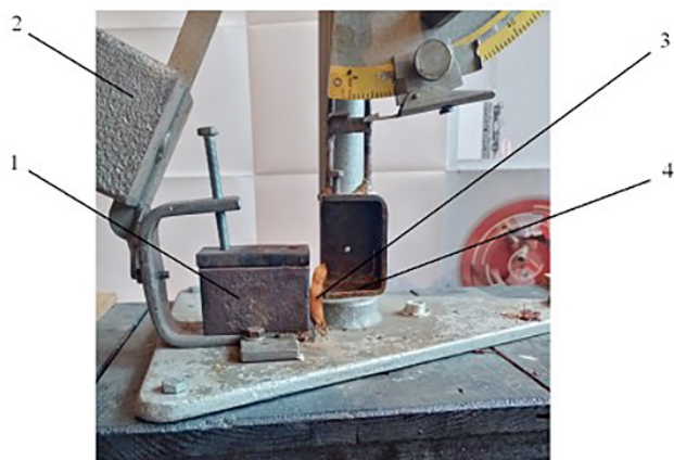
Fig. 2. Measurement of the consumed energy for shattering of a single soybean pod
