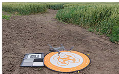
Fig. 1. Photo of DJI Mavic 2 Pro equipped camera MAPIR Survey3W_RGN
