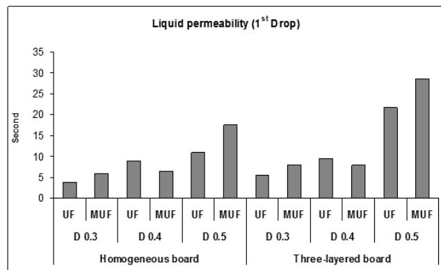
**Fig. 4. Liquid permeability of 1<sup>st</sup>-Drop (second) for the 12 treatments in the present study (UF = Urea Formaldehyde resin; MUF = Melamine Urea Formaldehyde resin; D = Density)**
