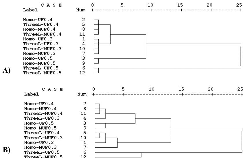
**Fig. 7. Cluster analysis of the 12 treatments based on specific gas permeability and the two liquid permeability of 1<sup>st</sup>-Drop and 50-mm lowering times (A), and based on specific gas and liquid permeability and noise reduction coefficients at the two 500 and 2000 Hz frequencies (B)**
