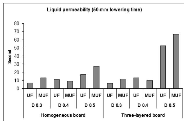
**Fig. 5. Liquid permeability of 50-mm lowering time (second) for the 12 treatments in the present study (UF = Urea Formaldehyde resin; MUF = Melamine Urea Formaldehyde resin; D = Density)**
