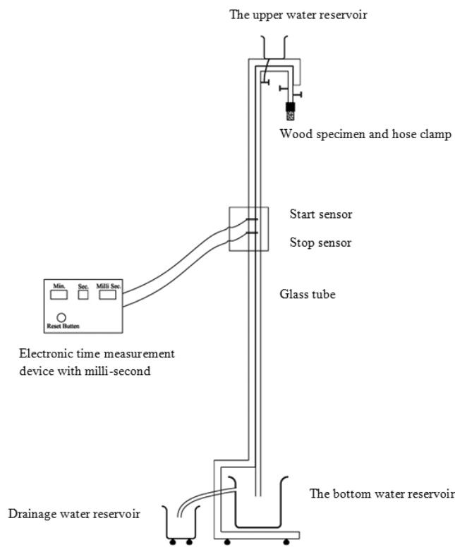
**Fig. 1. The overview of the gas permeability apparatus equipped with milli-second precision electronic time measurement device (USPTO No. 8,079,249 B2; Pub No. 2010/0281951) (Approved by The Iranian Research Organization for Scientific and Technology under certificate No. 47022)**
