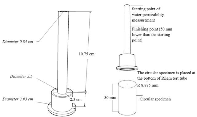
**Fig. 2. Liquid permeability measurement apparatus (Rilem test tube)**
