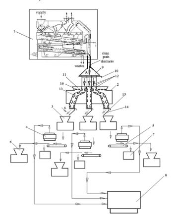
Fig. 1. Air-sieve grain-cleaning machine design
