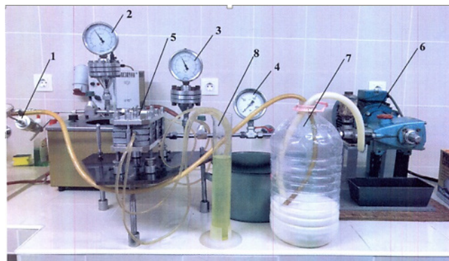
Fig. 1. Scheme of a laboratory equipment with a replaceable plate and frame membrane module: 1 – valve; 2, 3, 4 – manometers; 5 – replaceable plate and frame membrane module; 6 – pump; 7 – tank for initial solution; 8 – cylinder for permeate
