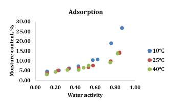
Fig. 2 Sorption isotherms of the mixture for the adsorption process at different water activities (aw) and temperatures t (°C).
