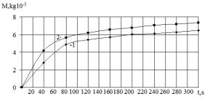
Fig. 4. Comparative analysis of the precipitate obtained: 1 – without using ultrasonic vibrations, the oil filtration temperature is 55°C; 2 – use of ultrasonic vibrations. Sonication mode: oil temperature 55°C with 1.3 kW ultrasonic vibration, ultrasonic wave frequency 120 kHz
