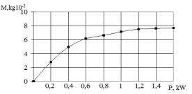
Fig. 5. Determine the filter cake for 200 seconds at an oil temperature of 55°C and change the force of ultrasonic vibrations
