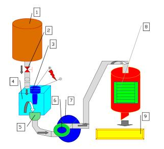
Fig. 1. Experimental installation for cleaning sunflower oil with ultrasonic field:
