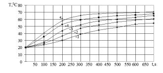
Fig. 2. Determination of the oil filtration temperature when changing the frequency of the ultrasonic oscillations of the power supply: 1 - 24 kHz, 2 - 50 kHz, 3 - 75 kHz, 4 - 115 kHz, 5 - 130 kHz
