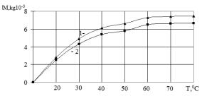
Fig. 6. Determination of sediment for 200 seconds filtration and change of oil temperature:
