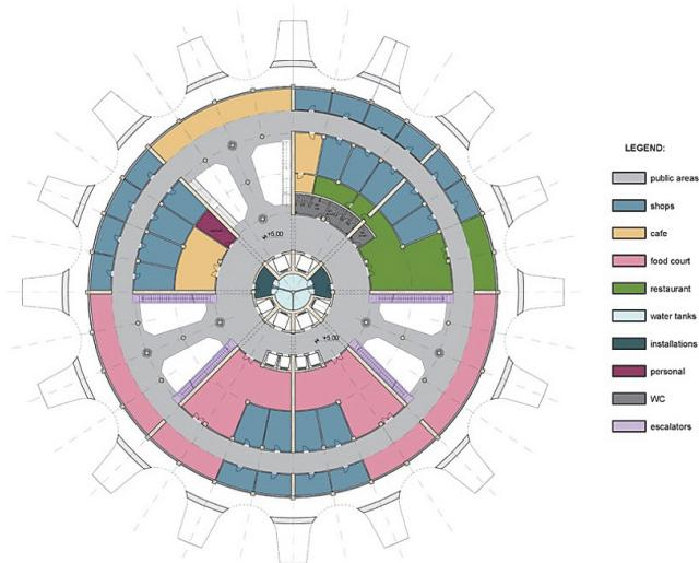
**Fig. 4. Architectural plan of the second floor (level 34.50 m) (Aleksandrov et al., 2014b)**
