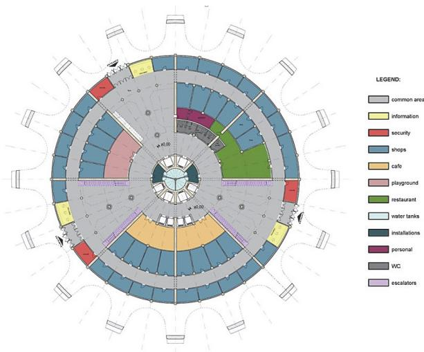
**Fig. 5. Architectural plan of the ground floor (level 0.00 m)**
