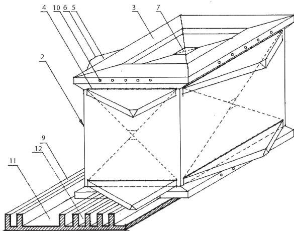
**Fig.12. Refrigerator for fruits and vegetables. General view. Patent for invention "Built-up refrigeration chamber". BG63644 (B1) (Aleksandrov, 2002)**
