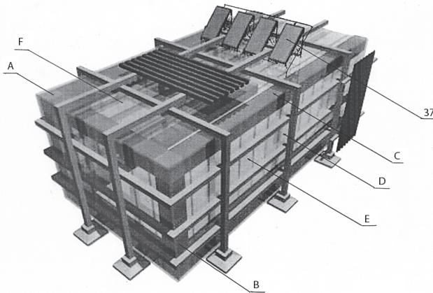
**Fig. 16. Refrigerator for fruits and vegetables. Elevation. System for solar heating of cooling chamber with positive temperatures.” (Reg. № BG111658 (A); Patent № BG 66742); (Aleksandrov, 2013b; 2018b)**
