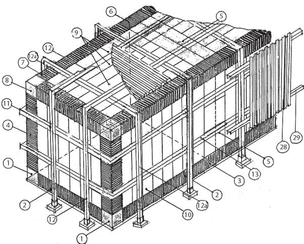
**Fig. 14. Refrigerator for fruits and vegetables. General view. „Moveable cold storage chamber for positive temperatures”. (Reg. № BG111651 (A); Patent № BG 66823); (Aleksandrov, 2013a; 2018a)**
