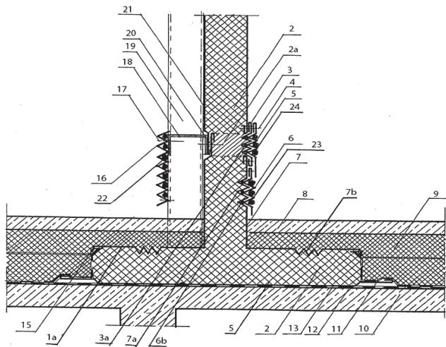
**Fig. 17. Refrigerator for fruits and vegetables. „T“-shaped joint. „System for solar heating of a cooling chamber with positive temperatures”. (Reg. № BG111658 (A); Patent № BG 66742); (Aleksandrov, 2013b; 2018b)**
