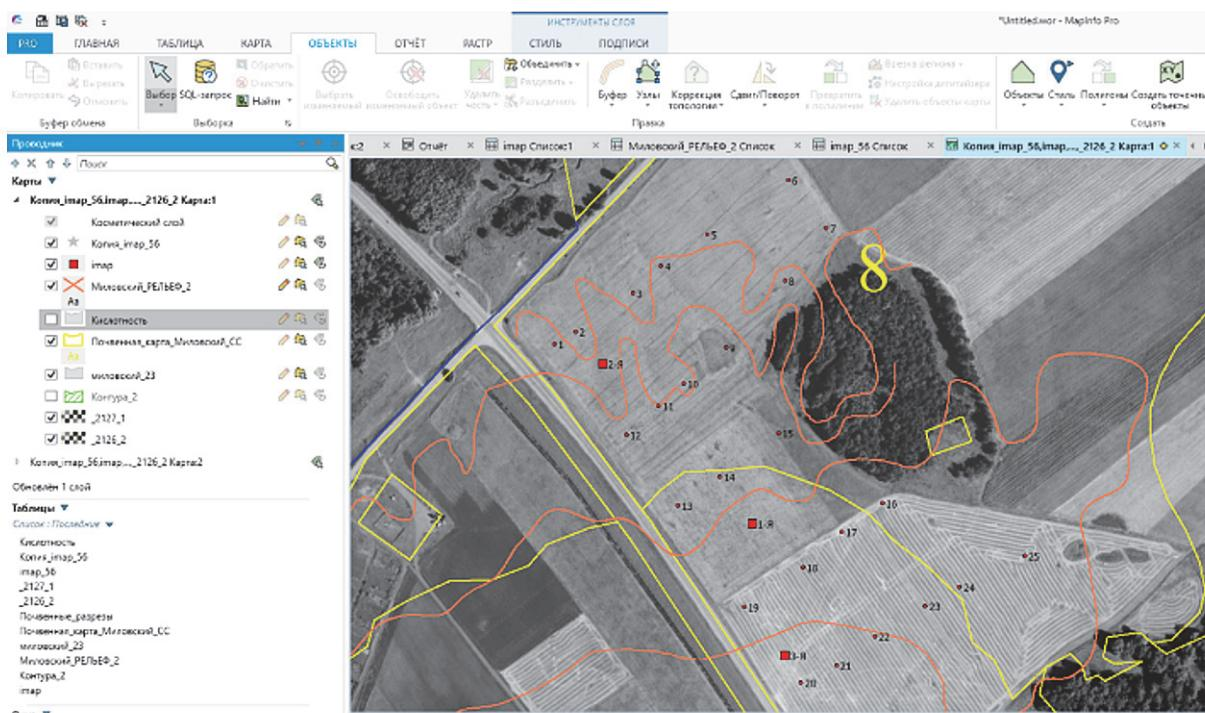
Fig. 4. Application of sampling points on a cartographic base
