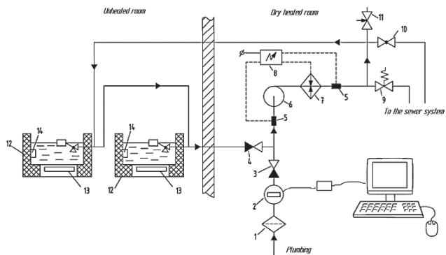
**Fig. 4. Schematic diagram of the circulating heating installation of water in the auto drinkers**
