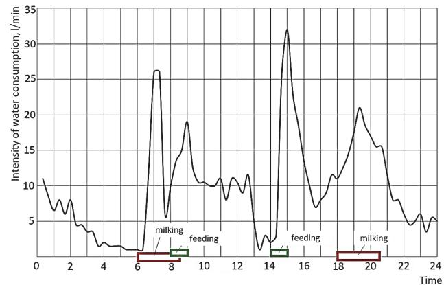
**Fig. 7. Intensity of water consumption in the barn**
