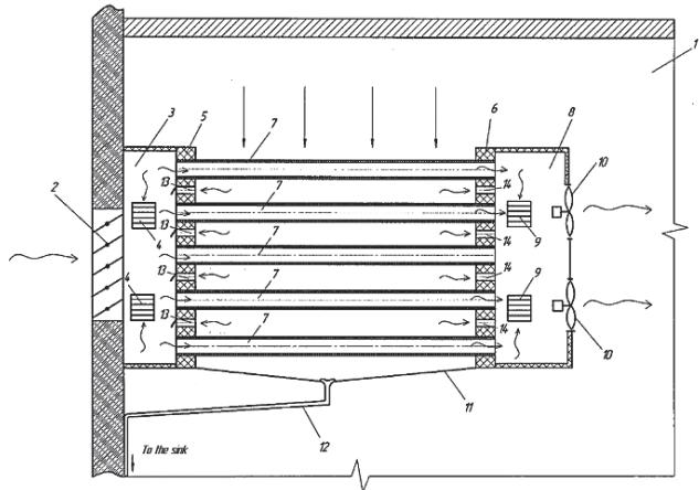
**Fig. 3. Scheme of air supply and recirculation unit**
