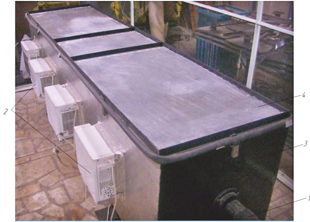
Fig. 2. General view of the process unit: 1 – shaft for rotation of the sawn timber along the axis in the chamber, 2 – magnetrons, 3 – the unit housing, 4 – steel wire cover
