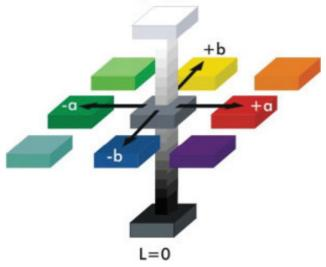
Fig. 1. Chromaticity diagram of the CIE system
