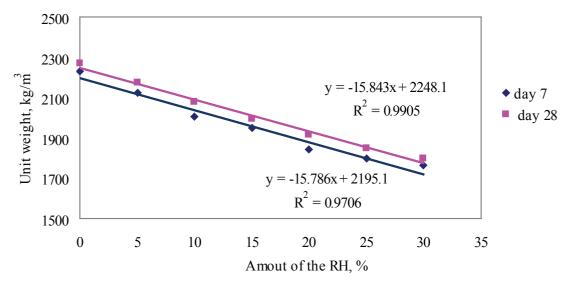
Fig. 2. The unit weight versus the amount of RH
