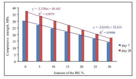
Fig. 3. The effect of RH on the compressive strength
