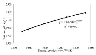
Fig. 6. The relationship between thermal conductivity and unit weight
