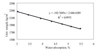
Fig. 5. The relationship between water absorption and unit weight
