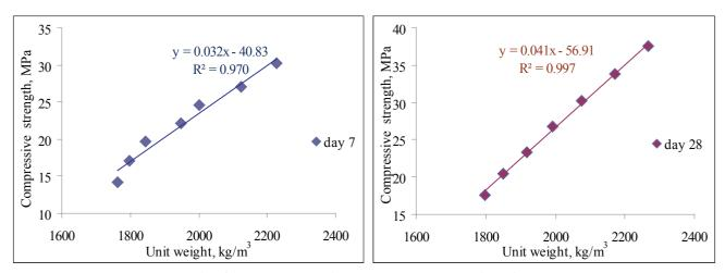
Fig. 4. The compressive strength versus unit weight
