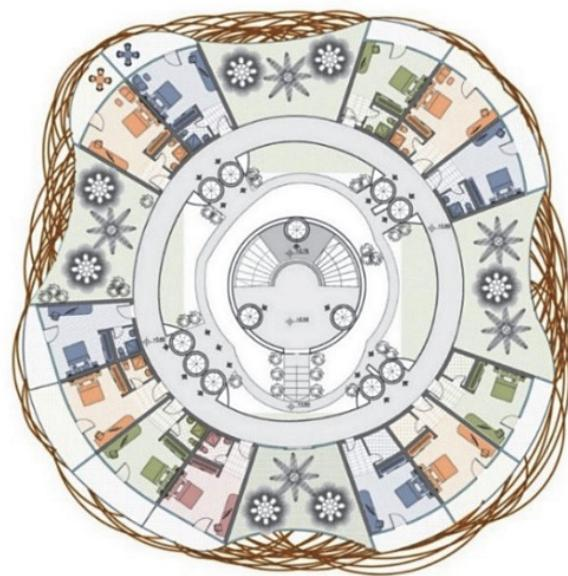
**Fig. 1. Plan of the floor with one capsule – there are three internal elevators and nine external elevators (Aleksandrov et al., 2014)**
