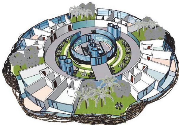
**Fig. 12. View of the floor with three internal elevators and four external elevators (Aleksandrov et al., 2014)**
