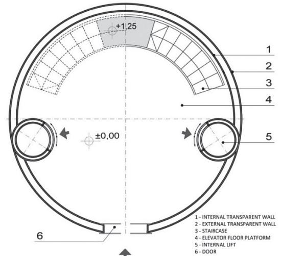
**Fig. 7. A panoramic vertical elevator with two peripheral internal lifts and two curved escalators or two curved staircases, transparent double external walls, vending machines and tables; dimensions 5.40 x 5.40 meters (Aleksandrov et al., 2014)**
