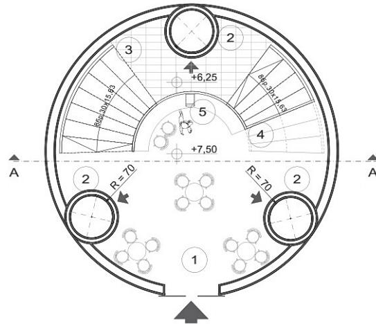
**Fig. 6. A panoramic vertical elevator with three peripheral internal lifts and two curved escalators or two curved staircases, transparent double external walls, vending machines and tables; dimensions 5.40 x 5.40 meters (Aleksandrov et al., 2014)**
