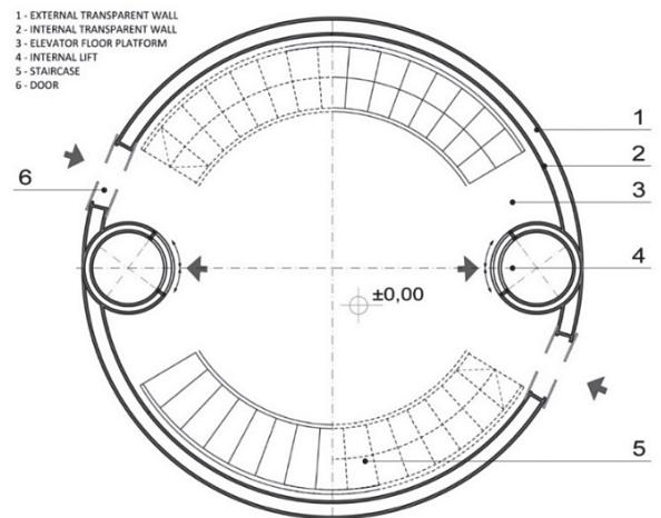
**Fig. 8. A panoramic vertical elevator with two peripheral internal lifts and two curved escalators or two curved staircases, transparent double external walls, vending machines and tables; dimensions 5.40 x 5.40 meters (Aleksandrov et al., 2014)**
