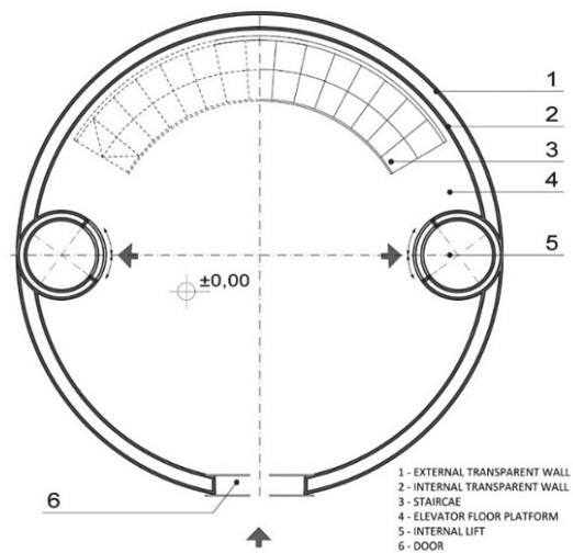
**Fig. 9. A panoramic vertical elevator with two peripheral internal lifts and one curved staircase, transparent double external walls, vending machines and tables; dimensions 5.40 x 5.40 meters (Aleksandrov et al., 2014)**
