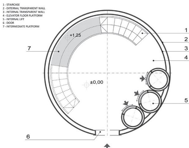
**Fig. 10. A panoramic vertical elevator with three peripheral internal lifts and two curved staircases, transparent double external walls, vending machines and tables; dimensions of 5.40 x 5.40 meters (Aleksandrov et al., 2014)**
