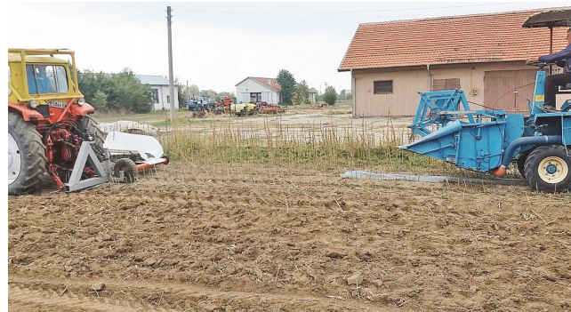
Fig. 6. Parallel determination of seed losses from grain harvester Wintersteiger and the developed device
