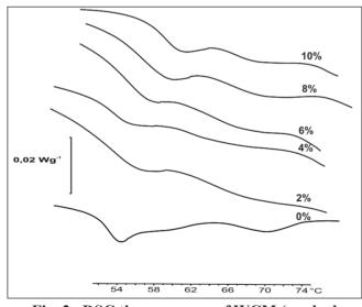
Fig. 2. DSC thermograms of WCM (washed chicken meat) stored for 360 days at -30°C as a function of mass fraction of maltose
