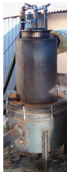
Fig. 2. The prototype of central heating boiler with rotating grate during testing
