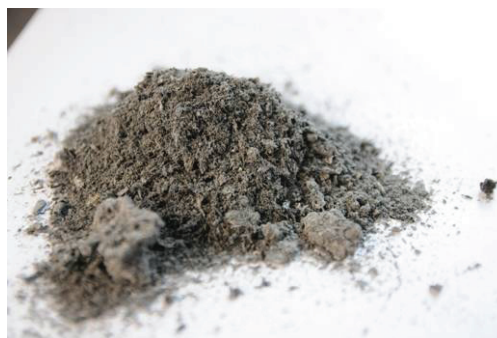
Fig. 5. The ash remaining after a briquettes portion burning. Source: Photo by Frackowiak
