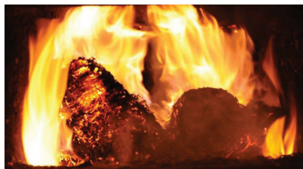
Fig. 4. View briquettes burning in the combustion chamber of the boiler at the time of the study
