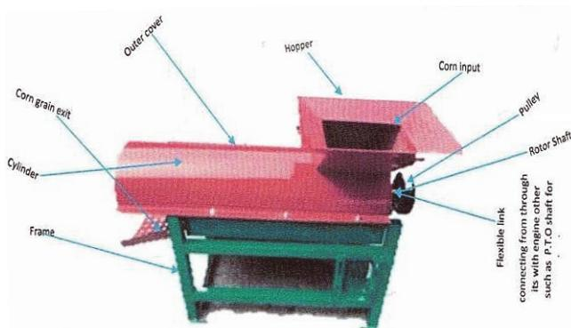
**Fig. 2. Machine (type Local Corn Sheller LCS-Irs2) used for corn shelling**
