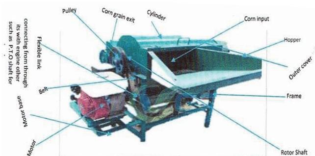
**Fig. 1. Machine (type Local Corn Sheller LCS-Irs1) used for corn shelling**
