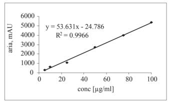
Fig. 2. Calibration curve of chlorogenic acid for HPLC test
