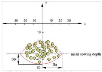
Fig. 2. Determination of seed distirbution area using with elipse criterion Sa: Standard deviation from row center of seed and Sb: Standard deviation of sowing depth
