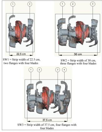
Fig. 1. Application of tillage strip widths by modification of rotary hoe.
