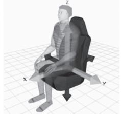
Fig. 1. Defining of orthogonal measuring directions on the tractor and the operator
