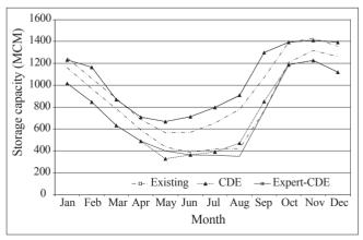
Fig. 6. Optimal rule curves of the Lampao reservoir (new and existing system)
