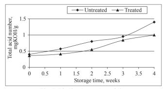
Fig. 7. Biodiesel samples acidity
