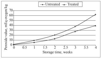
Fig. 8. Peroxide values of the samples of biodiesel
