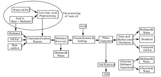
Fig. 2. Technological flow of obtaining biodiesel
