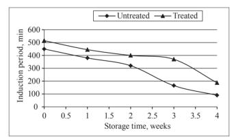
Fig. 6. Oxidation stability of biodiesel samples
