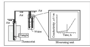
Fig. 4. Installation for the determination of stability in the biodiesel oxidation
