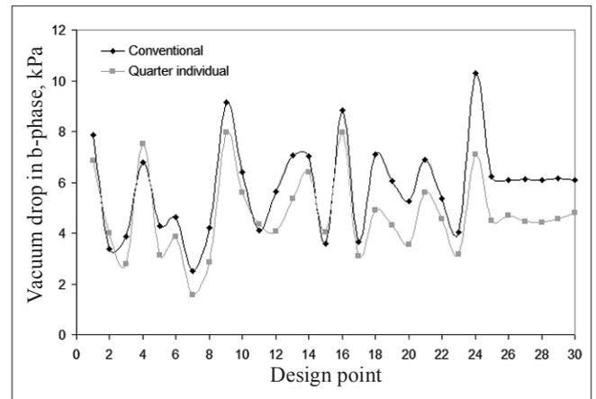
**Fig. 1. Vacuum drops in b-phase in conventional and quarter individual milking system based on the experiments conducted**
