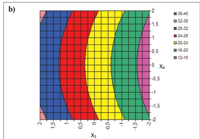
Fig. 4. Vacuum drops in d-phase in kPa a) conventional b) quarter individual milking system as a function of flow rate ( $X_3$ ) and pulsation rate ( $X_4$ ) (system working pressure,  $X_1$  and pulsation ratio,  $X_2$  are kept constant at the center, zero level)
