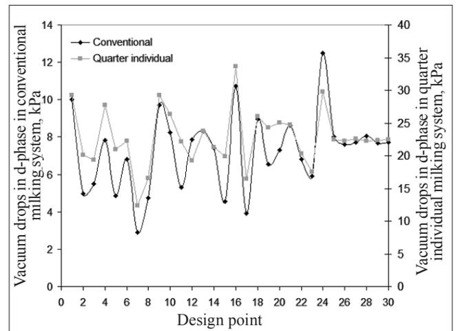
**Fig. 2. Vacuum drops in d-phase in conventional and quarter individual milking system based on the experiments conducted**
