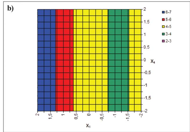
Fig. 3. Vacuum drops in b-phase in kPa a) conventional b) quarter individual milking system as a function of system working pressure ( $X_1$ ) and pulsation rate ( $X_4$ ) (pulsation ratio,  $X_2$  and flow rate  $X_3$  are kept constant at the center, zero level)
