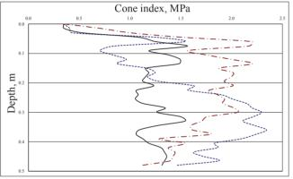
Fig. 5. The results of soil cone penetrometer resistance (cone index) in three measurement points (acquired using a sampling frequency of 2 Hz and an operating speed of 10 mm s<sup>-1</sup>) on the soil compacted after 20 tractor passes
