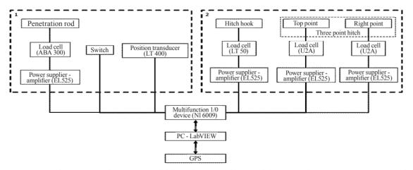
Fig. 3. The scheme of the system for data acquisition: 1) system for acquiring the soil cone penetrometer resistance;
