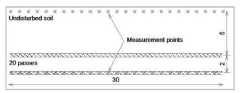
Fig. 4. The field experimental scheme (the distances are expressed in metres)
