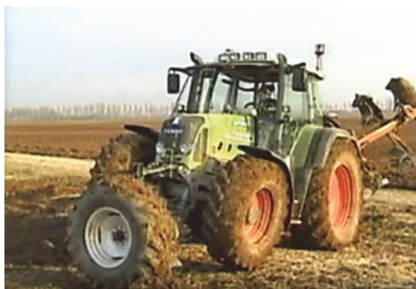
Fig. 1. Tractor with fifth wheel for making turns
