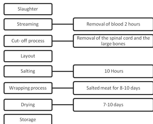
**Fig. 7. Technological process of production of Pasterma**
