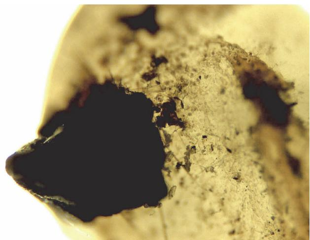
**Fig. 4. Sesame seed threshed by threshing apparatus of grain harvester**
