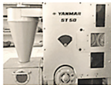
Fig. II. The machine (type Yanmar) which is used for hulling paddy
