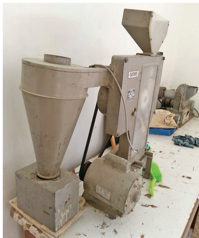
Fig. I. The machine (type Satake) which is used for hulling paddy
